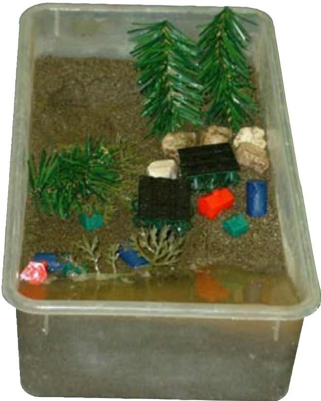
A designed landscape before and after water was applied. Note the destruction on the side of the box with few protective structures.
